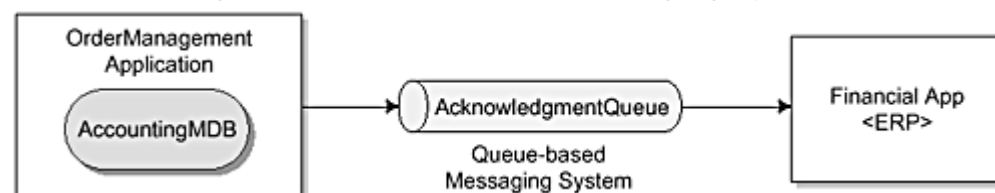
Figure 6.13. Queue-based Messaging System
